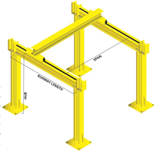
This manual top running crane is ideal for welding stations, assembly cells, machining centers and more. Bridge is designed to move easily under load. All structural steel, this crane is designed for heavy duty applications. Bridge lengths are 10, 15 and 20 ft. Bridge includes tagline. Standard heights under beam (HUB) are 12 and 14 ft. Runway lengths are 10, 15 and 20 ft lengths. Runways are easily expandable by simply removing the end stops—bolting beams to columns and replacing end stops .
