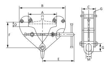
The eye beam clamp can be used as an anchor for various applications and for any type of construction. The zinc plated clamp screw assembly allows for easy adjustment of the clamp. This clamp features metric capacities that range from 1, 2, 3, 5, and 10 tons.
